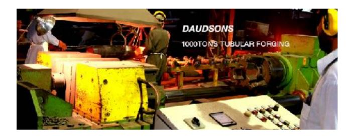
Daudsons Armoury (Pvt) Ltd has installed **TWO** State of the Art large capacity/Horizontal Forging Presses which are capable of handling Tubular Products requiring complex contouring and upsetting so as to give controlled variation in Wall Thickness and Variable Diameter.
